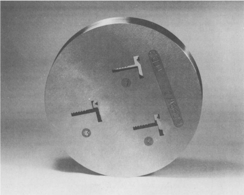
*Figure 13 - Multiple passages in one workpiece can be processed simultaneously.*
