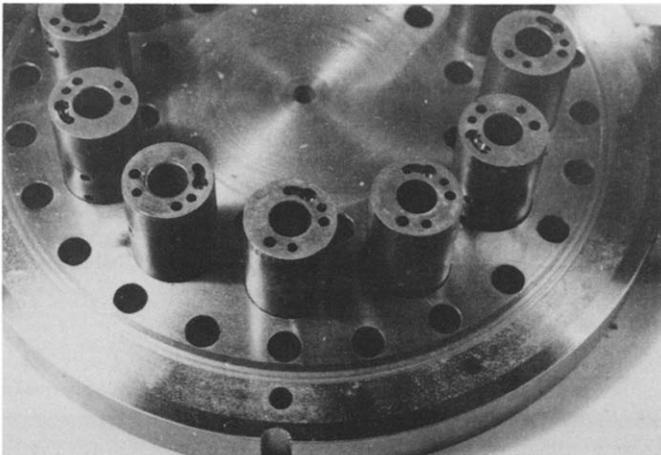
*Figure 7 - Twelve diesel fuel injector nozzles in one fixture are processed simultaneously.*
