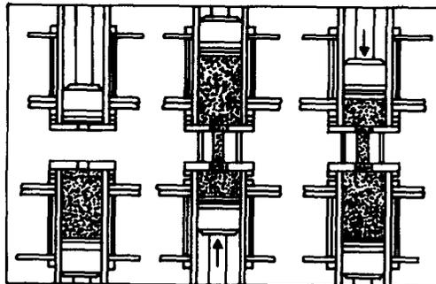
Figure 1 - Abrasive Flow Machining Process
